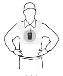
No close body blocking Partial RF absorption
