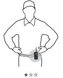
Partial close body blocking due to low position Partial RF absorption
